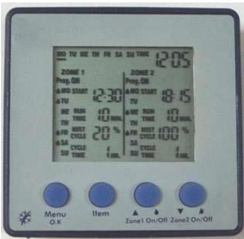
Or you can select 10~90%, if your RUN TIME set up 10mins and up. It has regular stops of 10 minutes during every section of RUN TIME. Otherwise, you only can select 50% or 100% when the RUN TIME set up value under 10mins.
